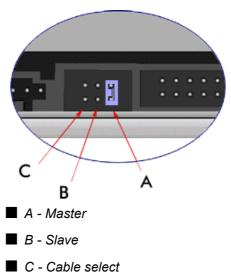
Figure 4 - 33 : Jumper settings (example)
